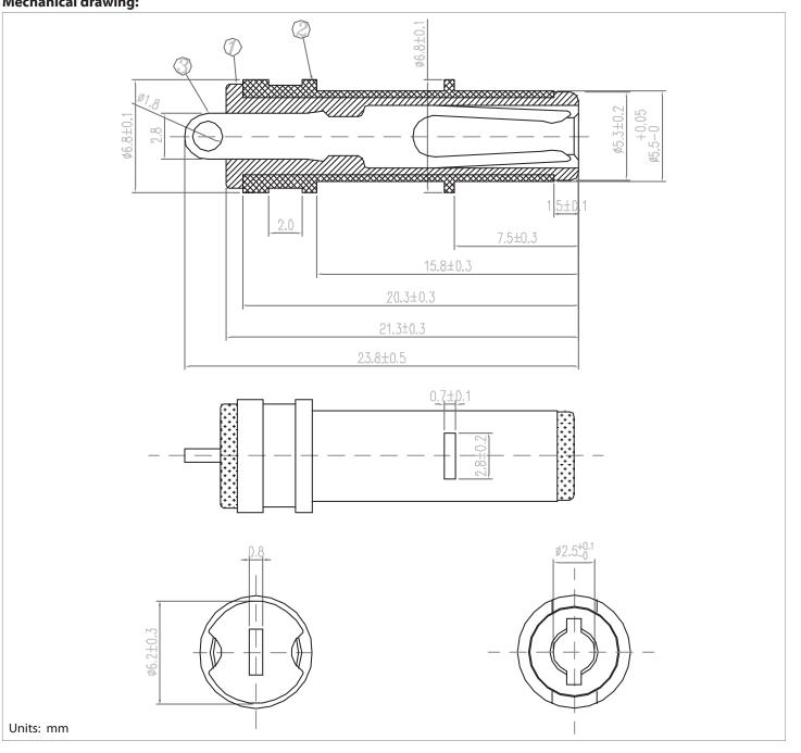
tolerance X: ±0.5 mm .X: ±0.3 mm .XX: ±0.05 mm applicable unless otherwise indicated in specification or on drawings **Initial** Date
