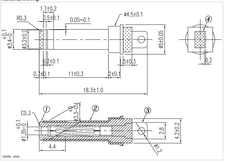
**tolerance** X: ±0.5 mm .X: ±0.3 mm .XX: ±0.05 mm applicable unless otherwise indicated in specification or on drawings
