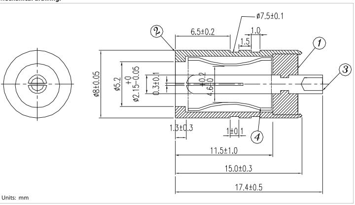
tolerance X:  $\pm 0.5 \, \text{mm}$  .X:  $\pm 0.3 \, \text{mm}$  .XX:  $\pm 0.05 \, \text{mm}$  applicable unless otherwise indicated in specification or on drawings
