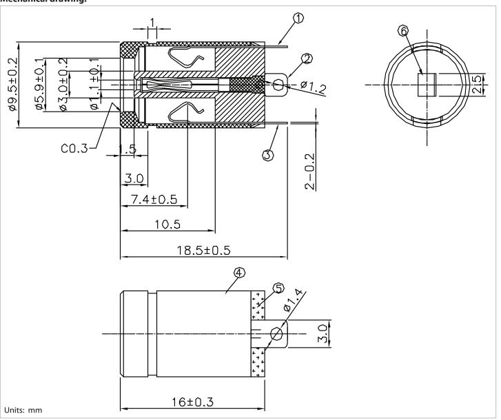
tolerance X:  $\pm 0.5 \, \text{mm}$  .X:  $\pm 0.3 \, \text{mm}$  .XX:  $\pm 0.05 \, \text{mm}$  applicable unless otherwise indicated in specification or on drawings
