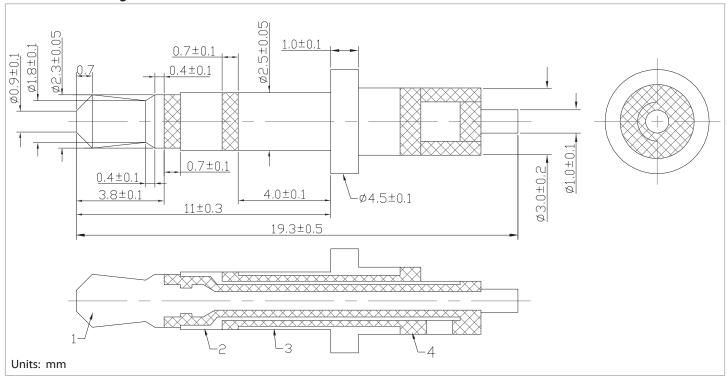
tolerance X:  $\pm 0.5 \, \text{mm}$  .X:  $\pm 0.3 \, \text{mm}$  .XX:  $\pm 0.05 \, \text{mm}$  applicable unless otherwise indicated in specification or on drawings
