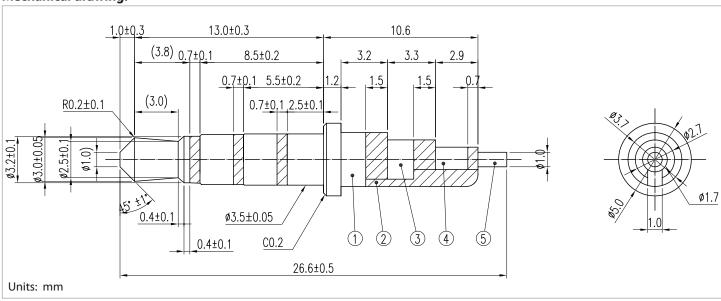
tolerance X: ±0.5 mm .X: ±0.3 mm .XX: ±0.05 mm applicable unless otherwise indicated in specification or on drawings
