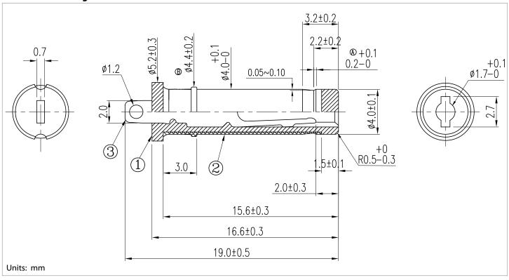
tolerance X:  $\pm 0.5 \, \text{mm}$  .X:  $\pm 0.3 \, \text{mm}$  .XX:  $\pm 0.05 \, \text{mm}$  applicable unless otherwise indicated in specification or on drawings
