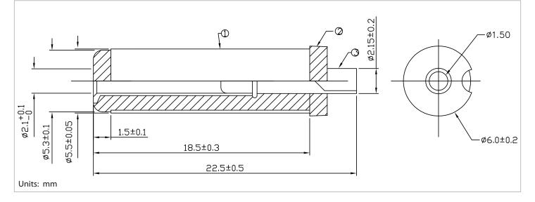
tolerance X: ±0.5 mm .X: ±0.3 mm .XX: ±0.05 mm applicable unless otherwise indicated in specification or on drawings
