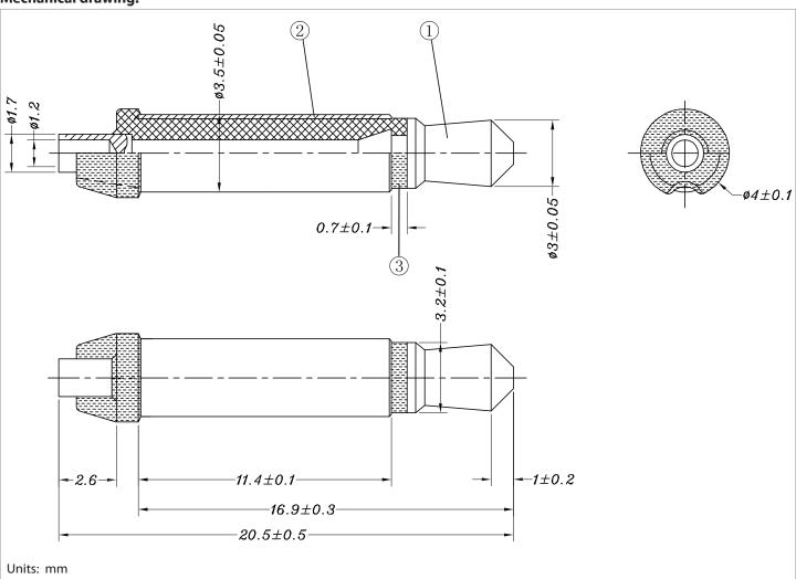
**tolerance** X: ±0.5 mm .X: ±0.3 mm .XX: ±0.05 mm applicable unless otherwise indicated in specification or on drawings
