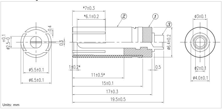
tolerance X: ±0.5 mm .X: ±0.3 mm .XX: ±0.05 mm applicable unless otherwise indicated in specification or on drawings
