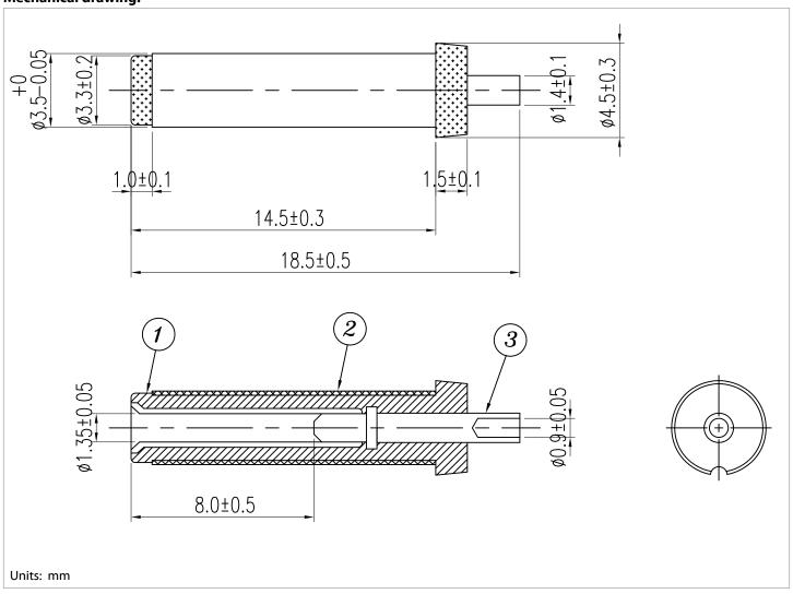
tolerance X:  $\pm 0.5$  mm .X:  $\pm 0.3$  mm .XX:  $\pm 0.05$  mm applicable unless otherwise indicated in specification or on drawings
