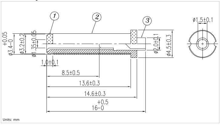
tolerance X:  $\pm 0.5$  mm .X:  $\pm 0.3$  mm .XX:  $\pm 0.05$  mm applicable unless otherwise indicated in specification or on drawings
