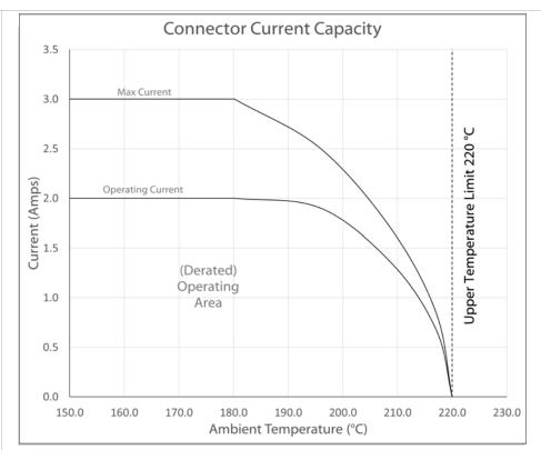
Testing based on IEC 60512-5-2. Max current curve generated with isolated test article under controlled environmental conditions, and does not take into account external factors such as housings, mating cables, or other
